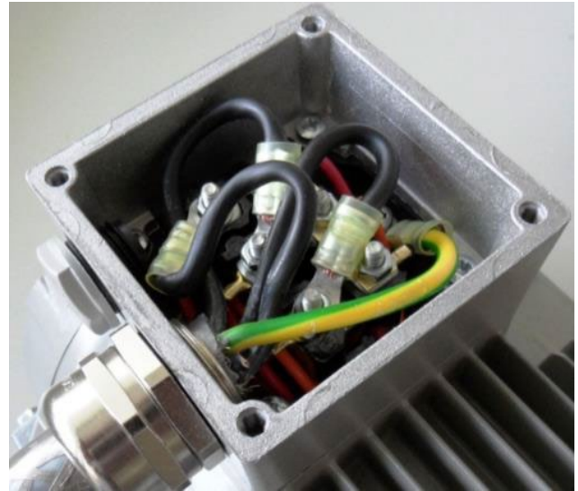
Fig. 23: Wiring on the motor connection box
