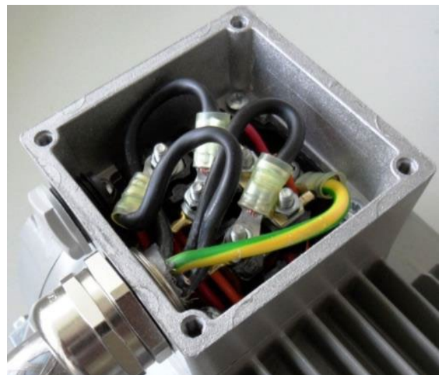
Fig. 30: Wiring on the motor connection box
