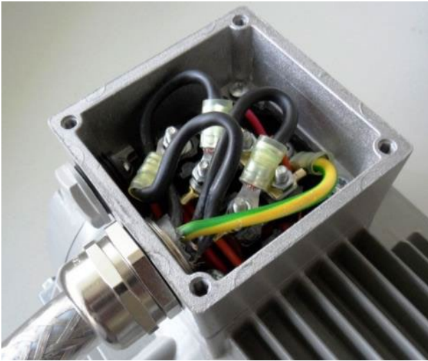
Fig. 24: Wiring on the motor connection box
